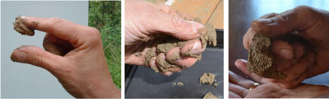
*Figure 7 Handling soil (left to right): a- Cohesive soil sticks; b- Sandy texture soil drops off after 12 mm (half inch); c- Loam soil with good cohesion drops off after >25 mm (an inch).*
