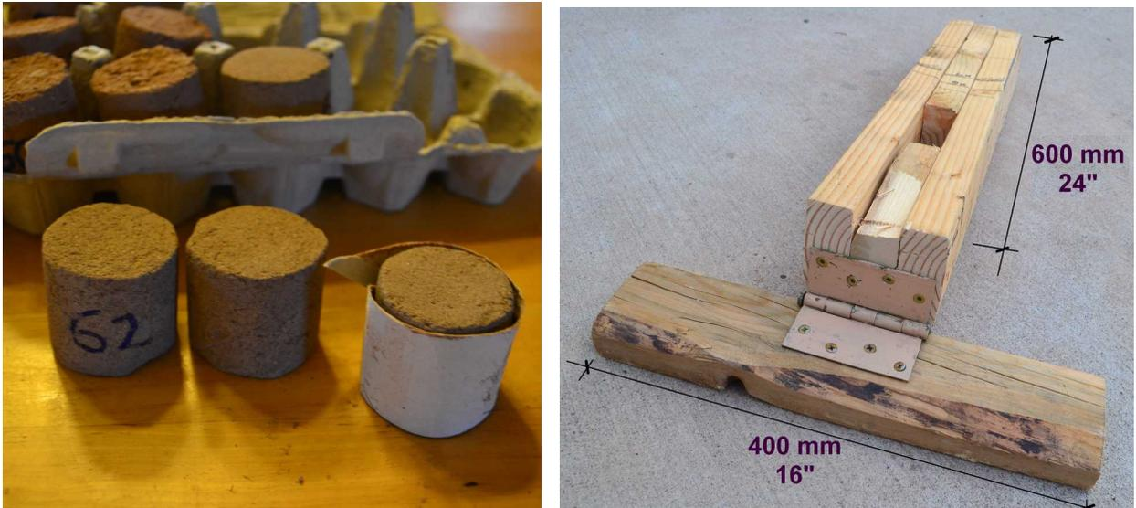
*Figure 10 Lever tests (left to right): a- Soil is finger-pressed into sections of toilet paper tube and dried; b- A simple wood lever can be used with buckets of soil and a 50 kg scale.*
