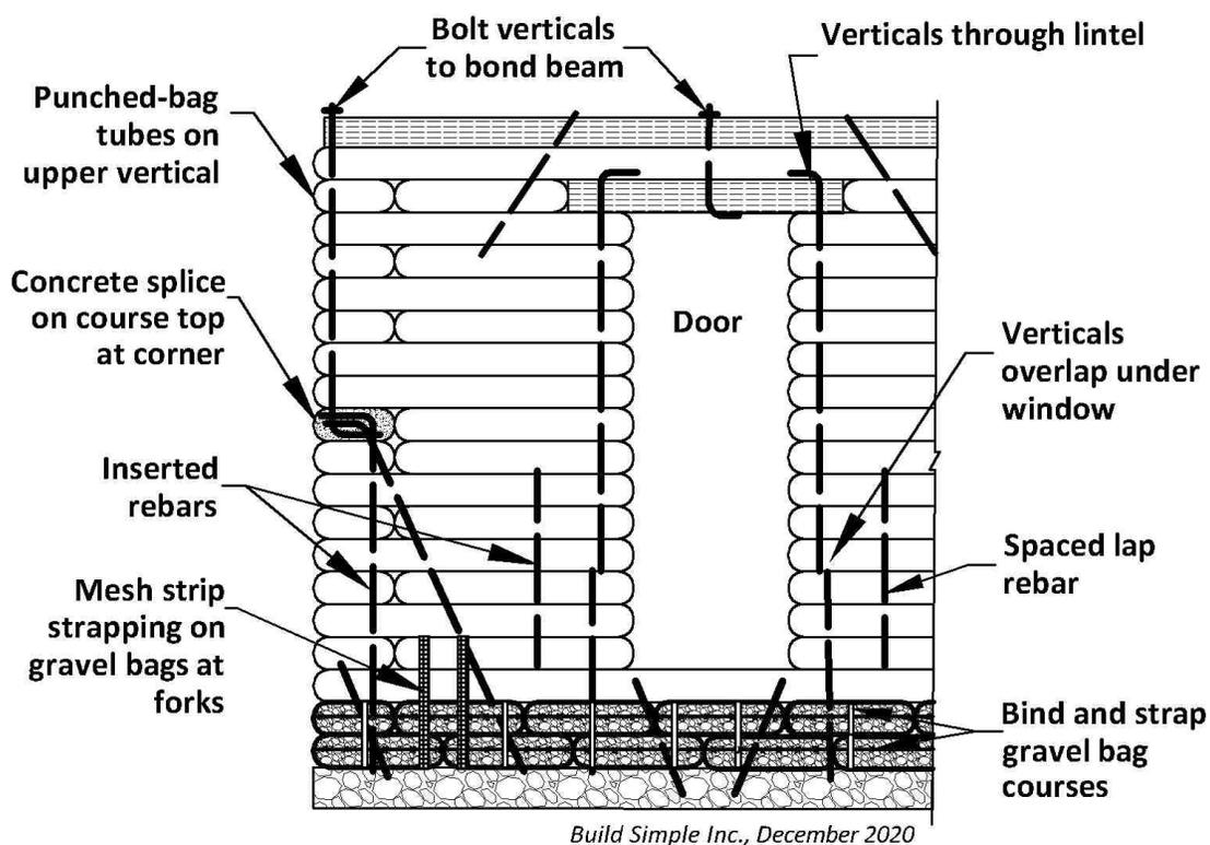
Figure 6: Improved reinforcement system for low seismic risk areas requires little Portland cement.
