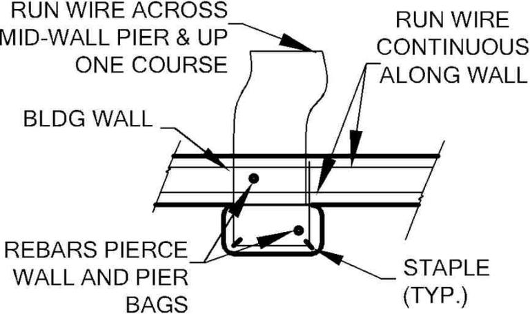
Figure 17 Barbed wire on piers should use a loop of wire woven to the next course.
