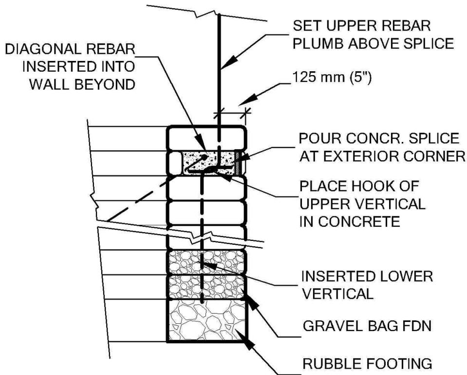
Figure 22 Concrete splice built on a course to connect rebars below and above.
