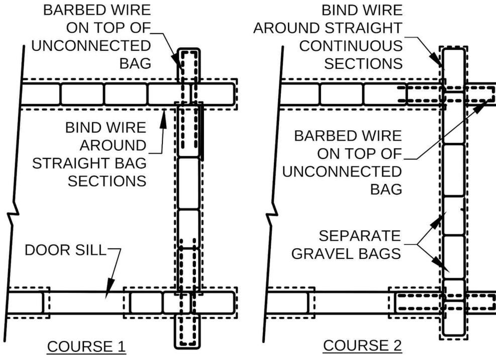
Figure 12 (left to right): a- Always bind the straight wall section that crosses a pier or intersecting wall first, then bind shorter sections next; b- Include buttresses in binding on alternate courses.
