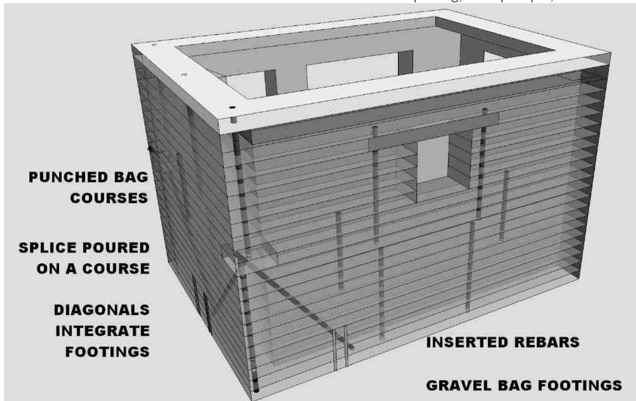
Figure 1: Strengthen corners by interconnecting upper and lower rebar to diagonals with a concrete splice poured during wall construction.
