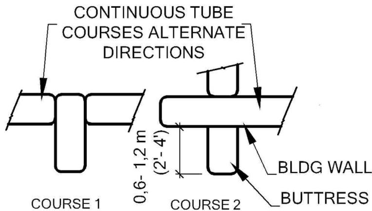
Figure 24: Continuous tubes and barbed wire unite walls to piers (left to right): a- Mid-wall buttress; b- Corner buttress tube layout.
