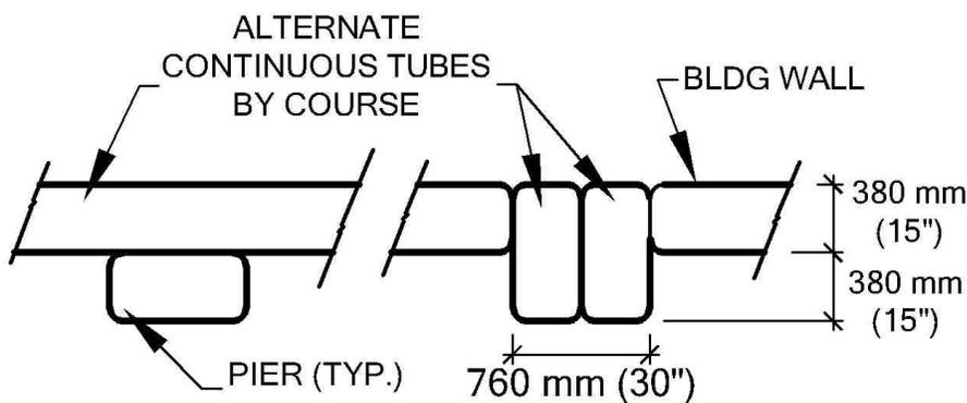
Figure 16 Piers integrated to the wall (left to right): a- Continuous tube lengths along the wall; b- Every other course interrupt the wall to run tubes across the pier and the wall.
