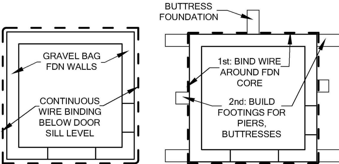
Figure 11 Bind to unify a building (left to right): a- with a simple shape; b- with buttresses bind main building core first, then lay footings for wall extensions.
