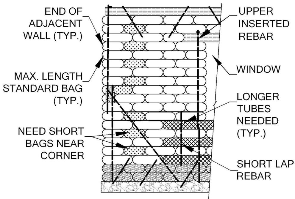
Figure 14: Bags limit rebar integration with wall material even when mixed with short tubes.
