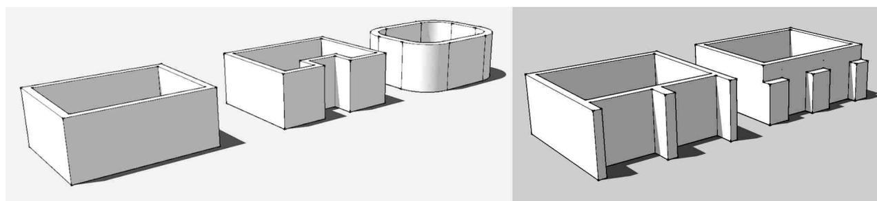
Figure 7 Structural wall elements (left to right): a- Corners on a rectangular building; b- Extra corners for nooks; c- Curved walls; d- Buttresses extending from walls; e- Piers that thicken walls.
