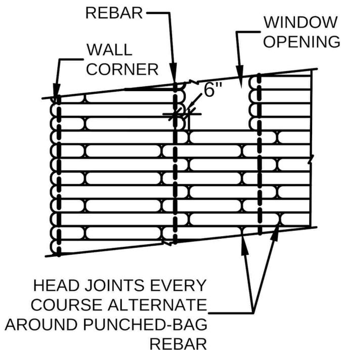
Figure 19: Punched-bag technique needs tubes starting on alternate sides of a vertical rebar to allow good overlap of tubes between courses.
