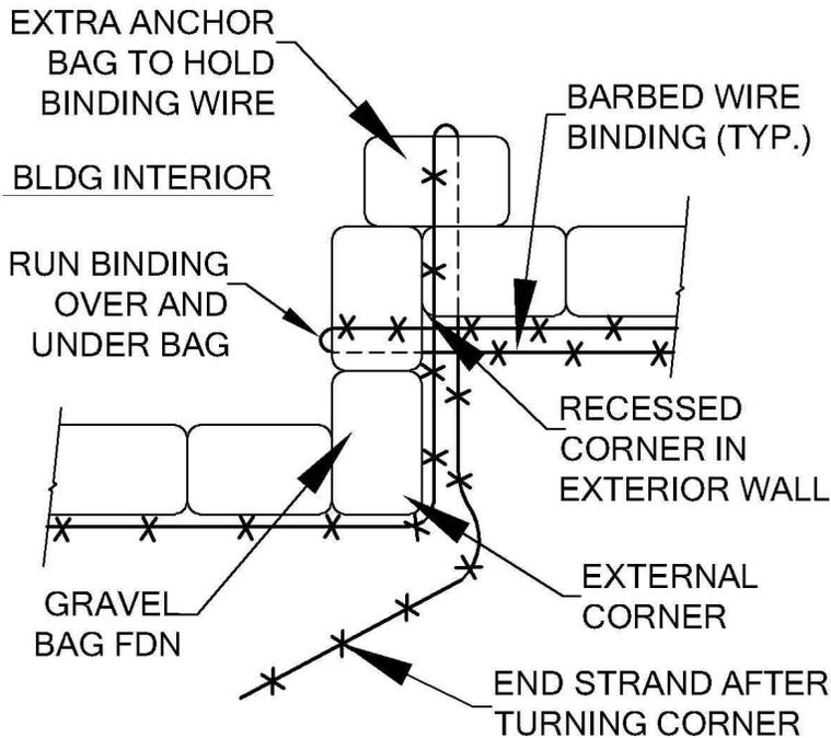
Figure 13: Start barbed wire at recessed corners by wrapping strands around a perpendicular bag.
