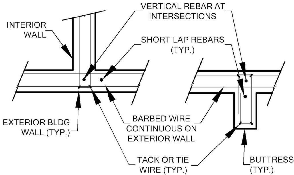
Figure 15 Barbed wire (right to left): a- at intersections crosses adjacent wall, b- at buttress loops.
