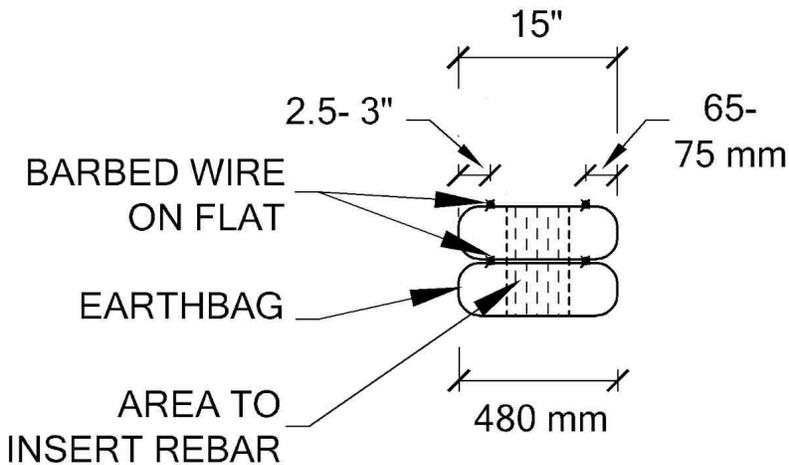
Figure 4 Barbed wire location on the flat course top near rounded course edges.
