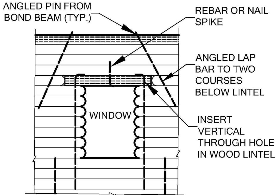
Figure 30: Vertical rebars adjacent to a window opening connect to the lintel.
