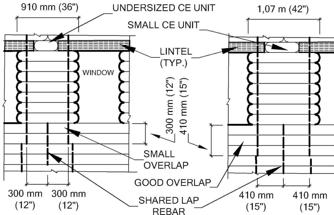
Figure 28: Spaced lap rebar dimensions (left to right): a- Minimum distance; b- Better distance.
