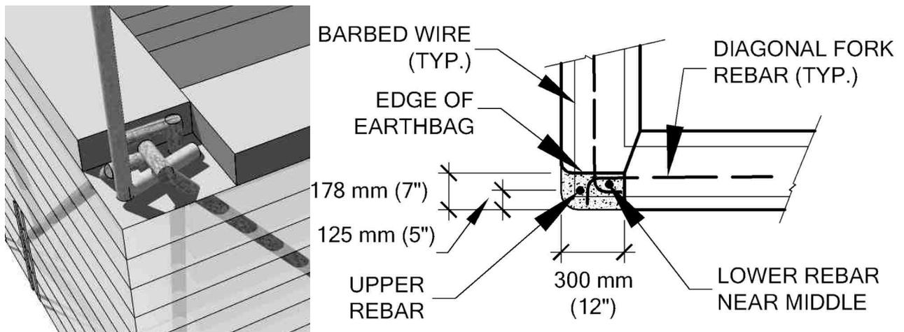
Figure 23 Spliced forks: a- hooks overlap at corner; b- Minimum size for a fork open splice.
