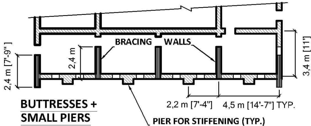
Figure 9: Bracing panels at 4,5 m (14'-9") spacing with piers between to stiffen walls.
