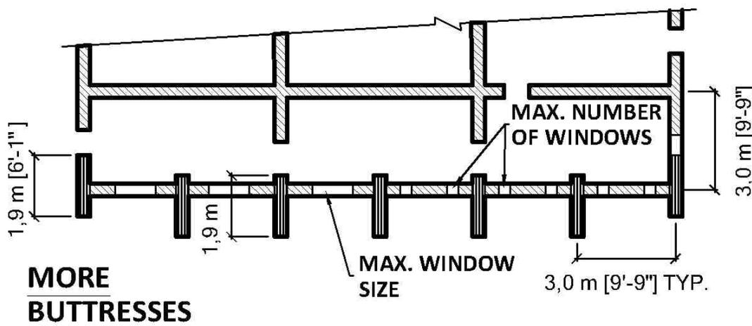
Figure 8 Bracing panels (above to below): a- A long supported right to left wall with few buttresses needs doorways far from wall corners; b- More buttresses allow doors closer to the supported wall.
