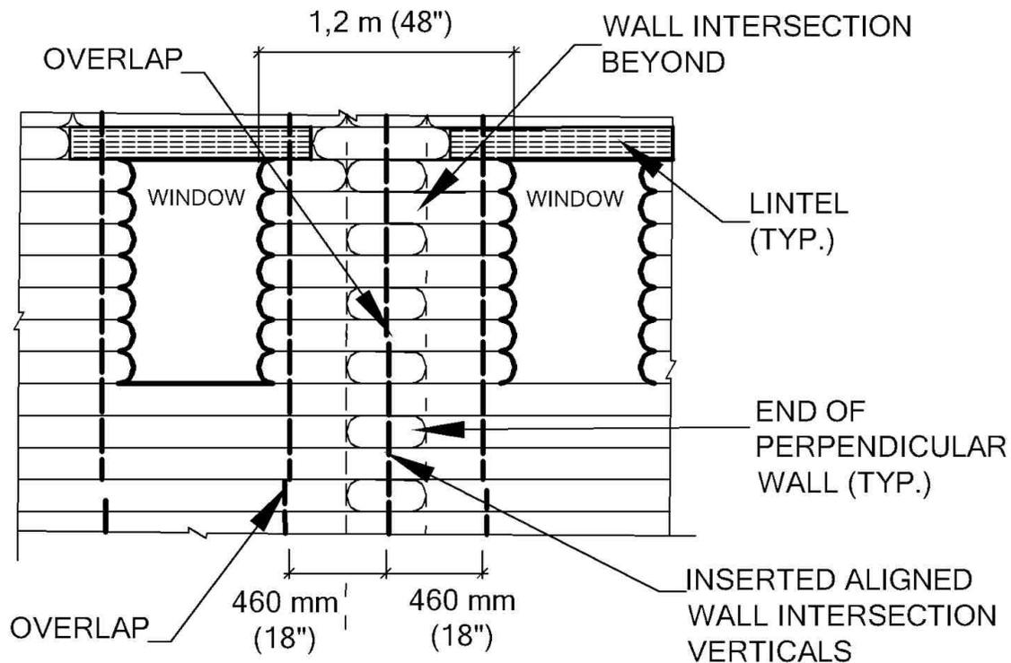
Figure 29: Use greater distance between openings when the area includes a perpendicular wall.
