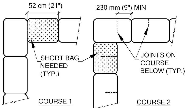
Figure 3: Shorter or longer bags are needed near corners and intersections for good running bond bag overlaps.
