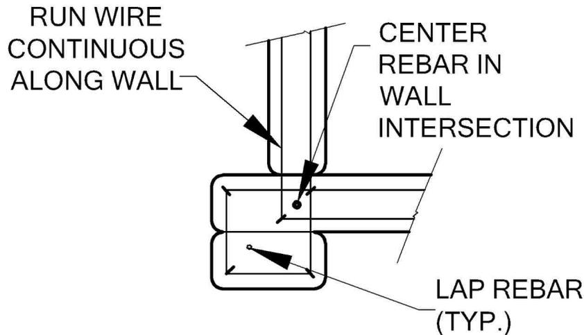
Figure 33 Corner pier barbed wire and rebar locations.
