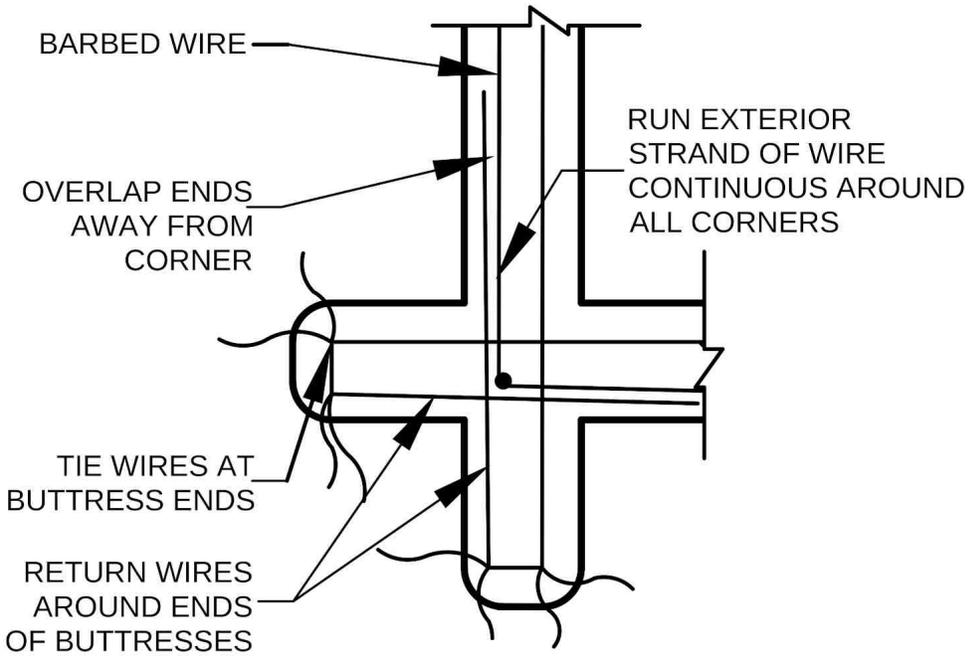
*Figure 25: Run external strand of barbed wire continuous around building and use interior strands to unite buttress to building walls.*
