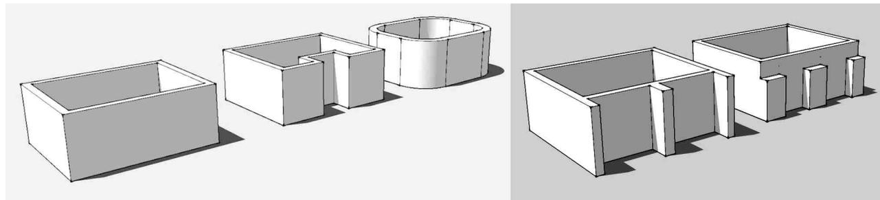
Figure 7 Structural wall elements (left to right): a- Corners on a rectangular building; b- Extra corners for nooks; c- Curved walls; d- Buttresses extending from walls; e- Piers that thicken walls.
