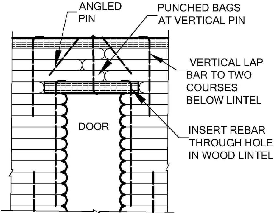
Figure 31: Vertical rebars adjacent to a door opening connect to the lintel.
