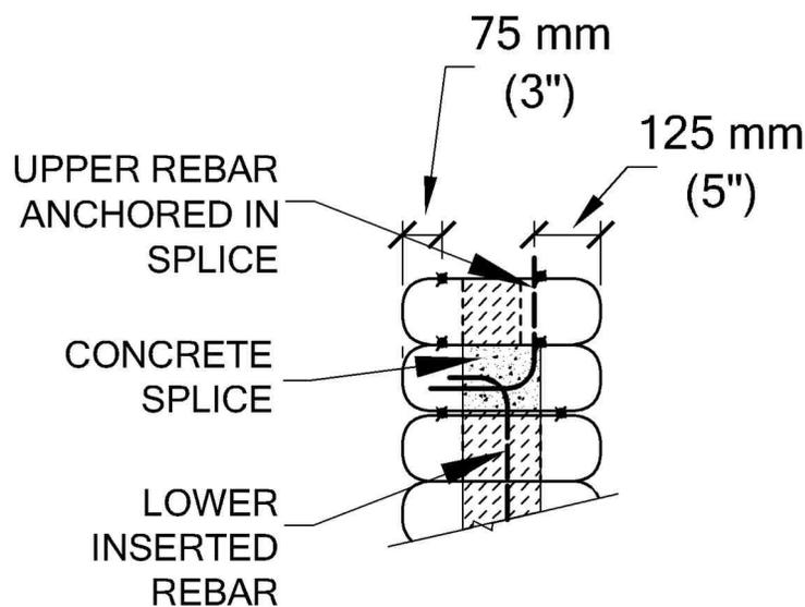
Figure 20: Barbed wire locations near punched-bag anchored rebar.
