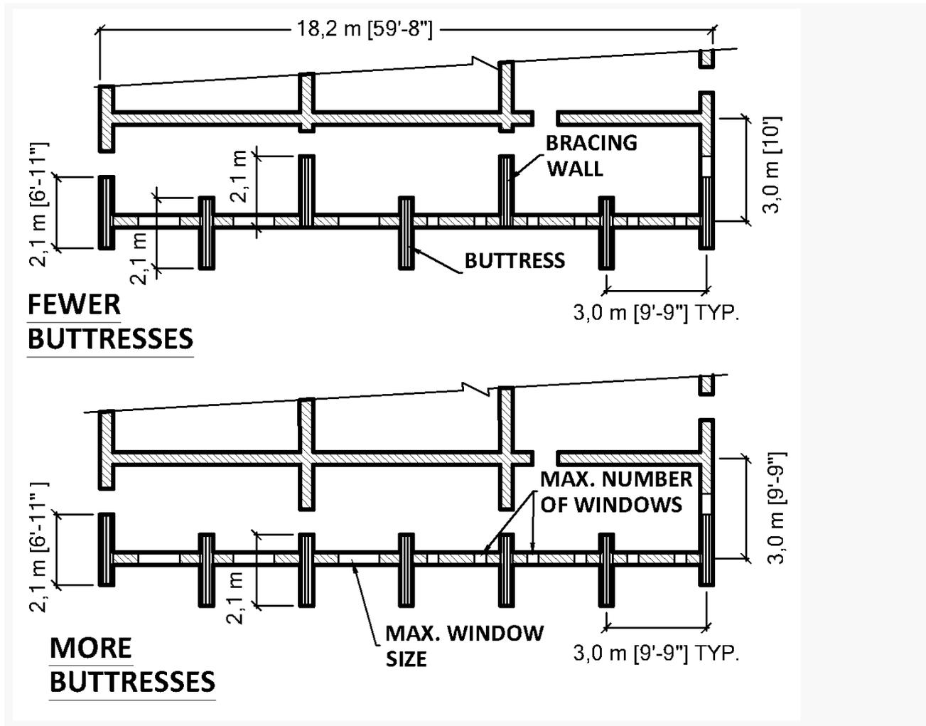
Figure 8 Examples of bracing panel sizes at 3 m (9'9") bracing line distances (above to below): a- Few buttresses and doorways distant from wall being braced; b- More buttresses and doorways closer to wall being braced.
