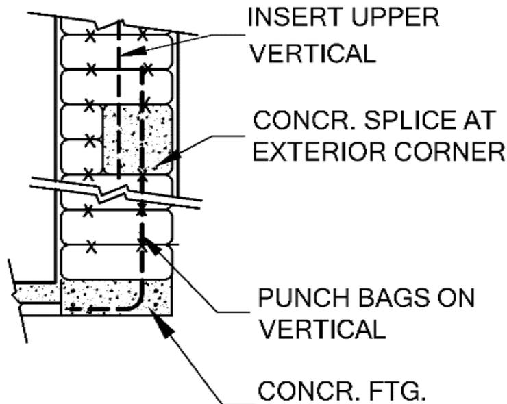
*Figure 28 An upper rebar inserted into a covered splice bag two courses high, then the sandbag is emptied and filled with concrete.*
