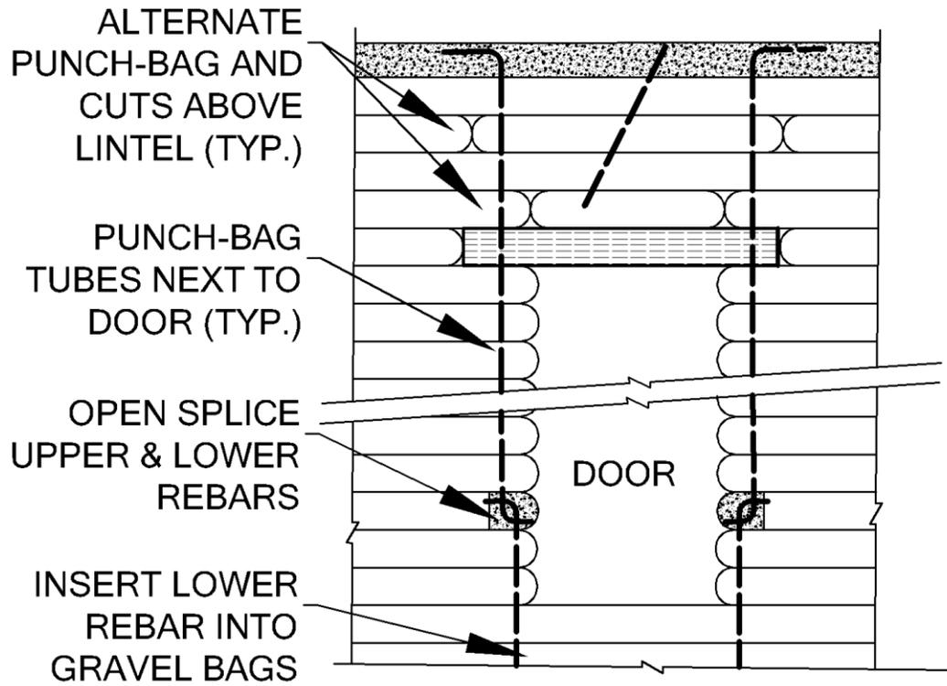
Figure 34: Splice vertical rebars next to doorways to provide vertical rebars extending below the door sill.
