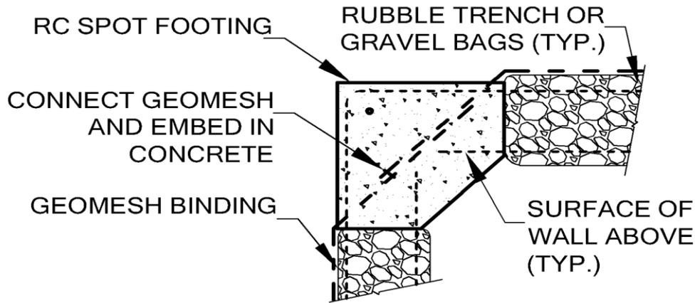
Figure 9 Geomesh embedded in spot footings at corners can confine adjacent gravel bag footings.
