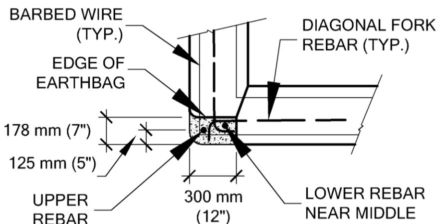
Figure 38 Reinforcement locations in a fork splice.
