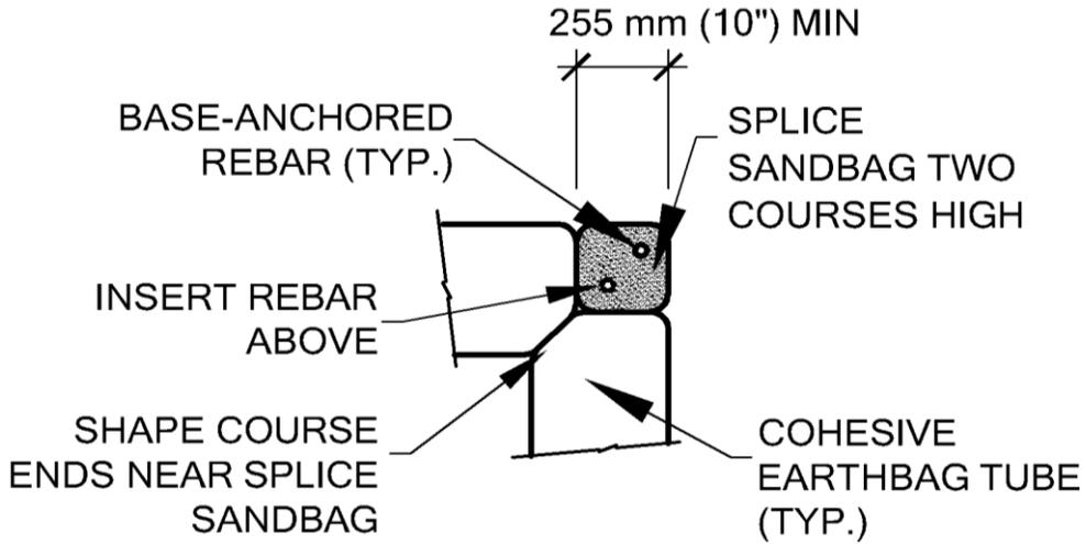
Figure 12 Covered splice sandbag location at mid-story height of external wall corners.
