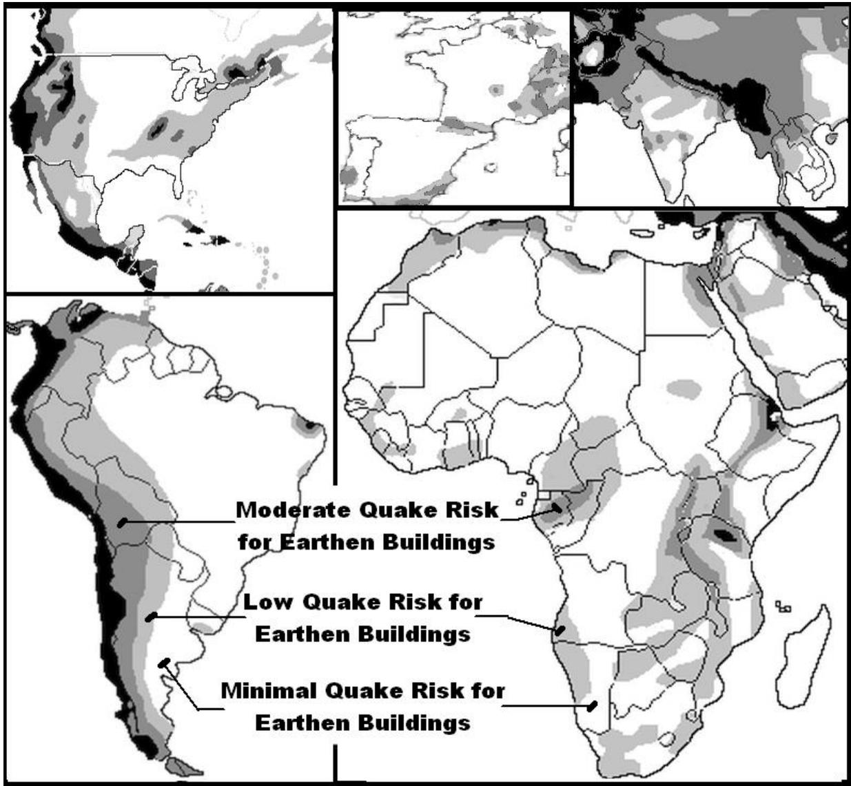
Figure 2: Approximate locations of earthquake risk relative to earthen wall strength.
