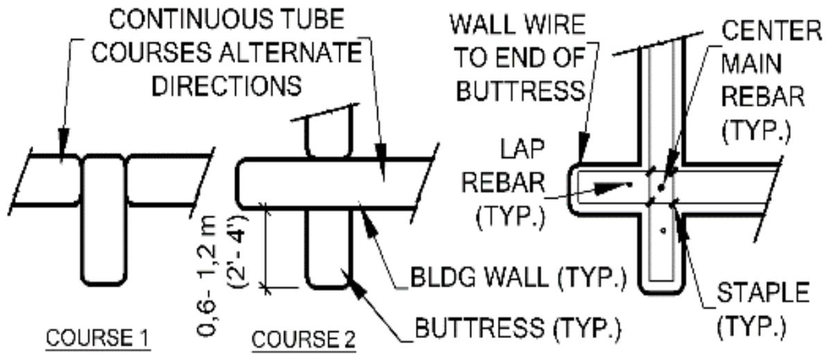
Figure 23: Continuous tubes and barbed wire unite walls to piers (left to right): a- Mid-wall buttress; b- Corner buttress tube layout; c- Corner buttress barbed wire and rebar.
