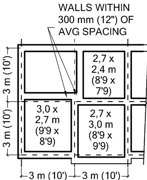
Corners and wall intersections closer together don't have to be as long as bracing wall panels spaced further apart. First step is to find out the average distance between walls and/ or buttresses in each major direction. Buildings do not need to be exact grids. Walls within 300 mm (12") of a bracing line act with it (Figure 7).
