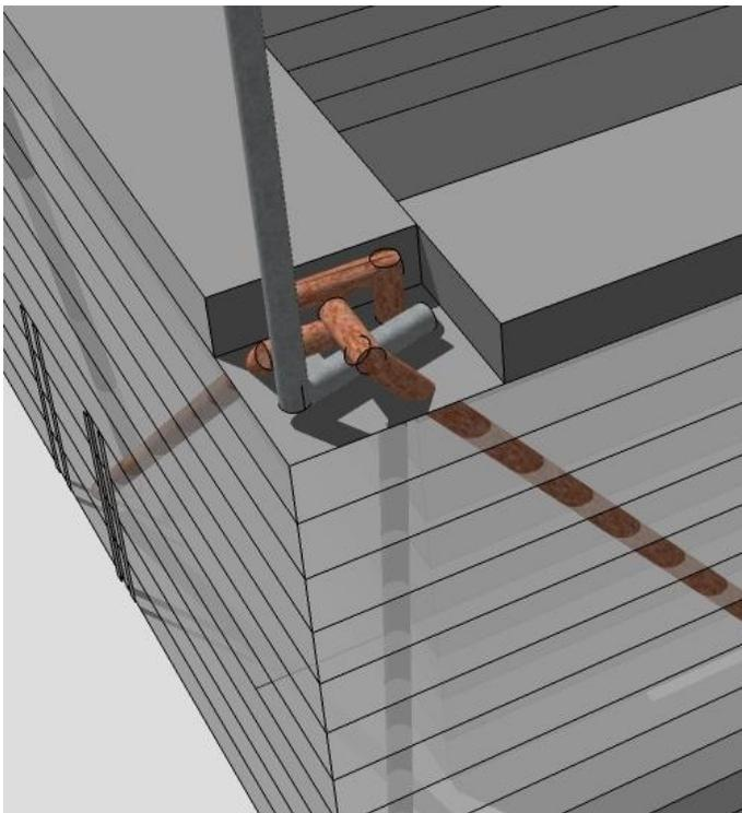
*Figure 37 Forming space for spliced forks at corners to connect diagonal and vertical rebars.*
