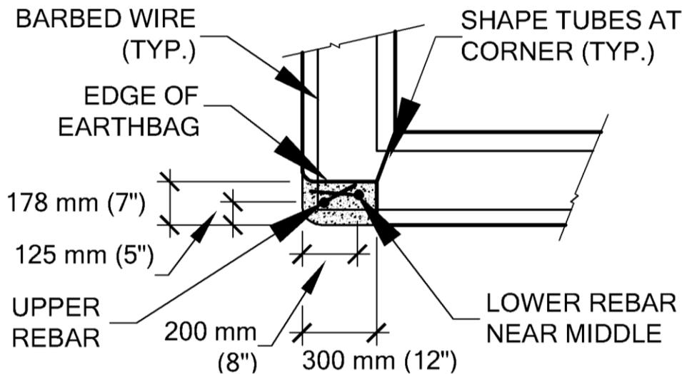
*Figure 27 Use a narrow gap for an open concrete splice to connect upper and lower rebars.*
