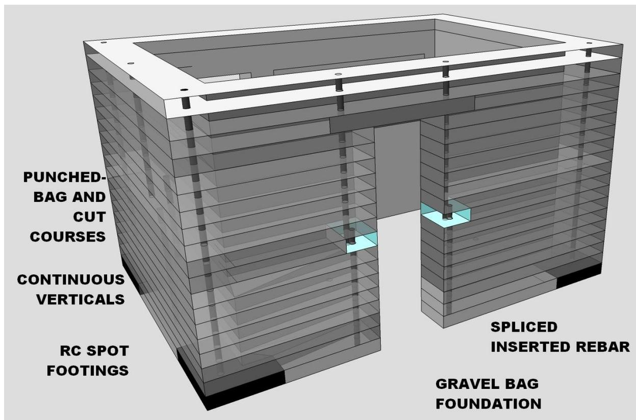
Figure 1: Strengthen corners with vertical rebar that is base-anchored in spot reinforced concrete footings. Insert spaced lap rebar at other locations on gravel bag foundations.
