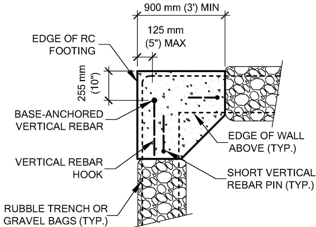
*Figure 11 Spot footing to anchor short vertical rebar that will use an open splice.*
