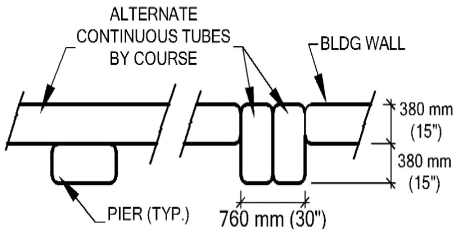
Figure 21 Piers integrated to the wall (left to right): a- Continuous tube lengths along the wall; b- Every other course interrupt the wall to run tubes across the pier and the wall.
