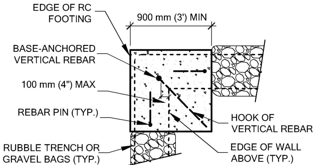
Figure 10 Spot footing to anchor long vertical rebar extending to the bond beam.
