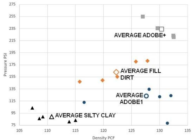
The four soil types shown at right are the four that were laboratory tested, with average results from 150- 370 psi.
