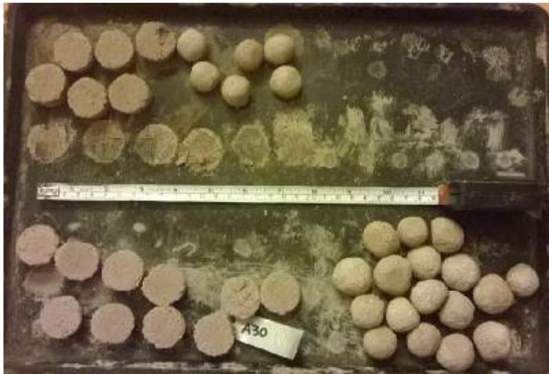
Left: 14 or more round samples and 16 bottle-cap samples were tested for each of the four soils during the second series of tests.
