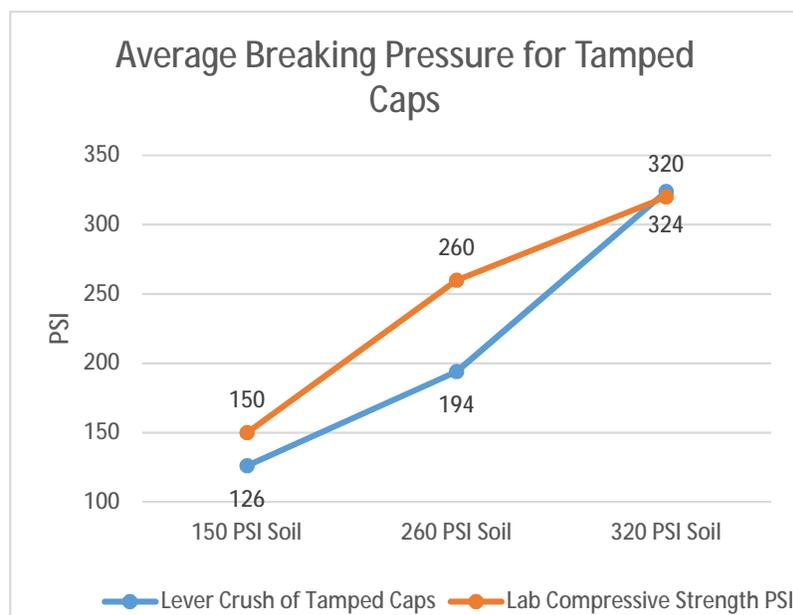
Balls of low and medium strength soils are close in performance. We recommend that soils tested under a shoe for Special/ NZ strength of 260 psi/ 1,8 MPa should be confirmed with a repeat test using wood.
