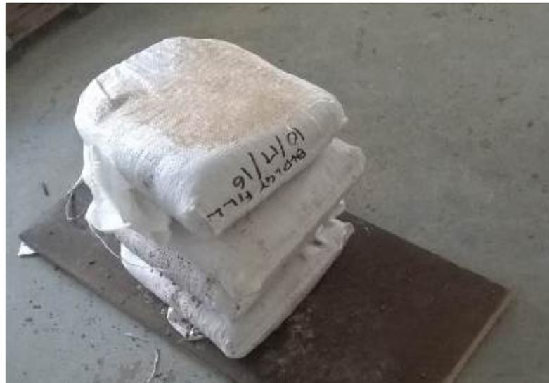
After one month lift the top two bags off to examine the bottom bag. Remove the bag. Does the earthen fill feel damp or cooler than the upper bags? If it does not feel damp or cooler, break the bottom sample in half. Does the interior feel damp or cooler? Does it have a uniform color or is it darker in the middle?
