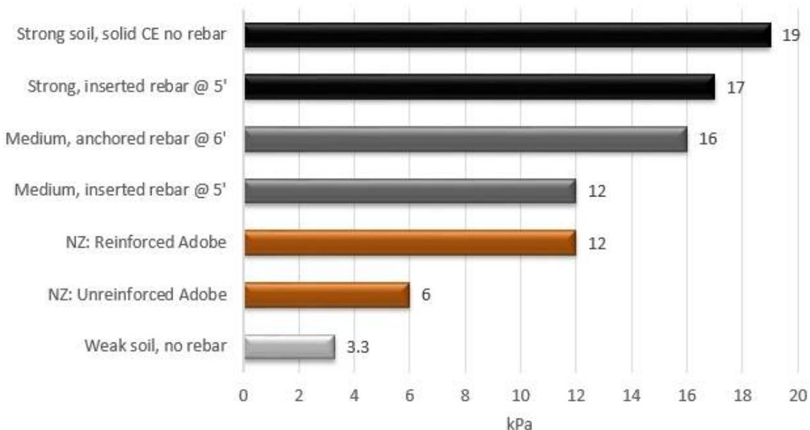
Good contained earth test results come from well-tamped walls with vertical strapping every 4 courses, overlapping by a course. Plaster embedded in mesh is important for earthen wall resistance to vibration. These tests used a cheap plastic fishnet, but tied it to the strapping that is also tied to the barbed wire. Chicken wire and cement stucco may increase wall strength also over these earth-plastered wall tests.
