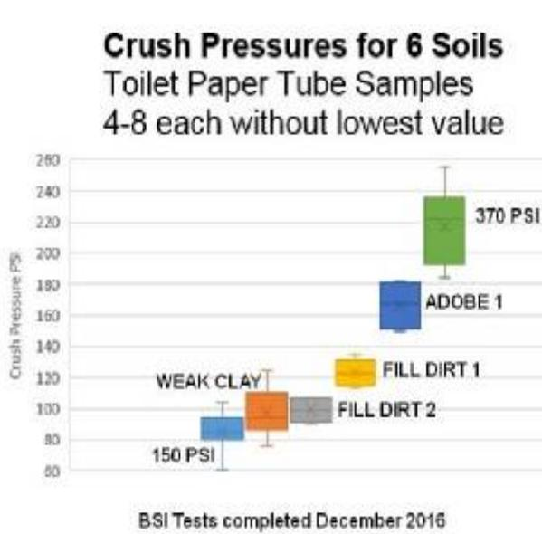
For most types of soil, the TP Tube crush tests shown at left had a small amount of variation.
