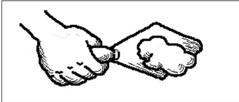
The plaster should be more thick than runny. A little should barely hold onto a trowel when it is held vertical.
