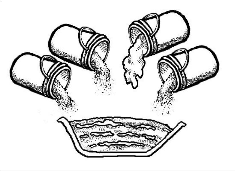
Spread the sand and putty in thin layers. Mix it together well with a hoe.
