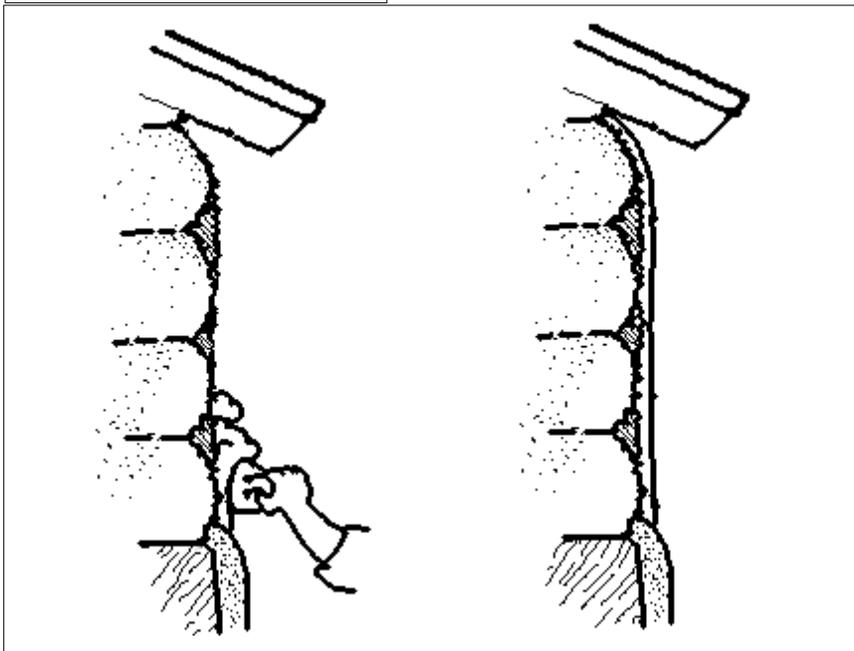
You can apply a thin layer of lime plaster. Start at the bottom on top of the cement stucco base.
