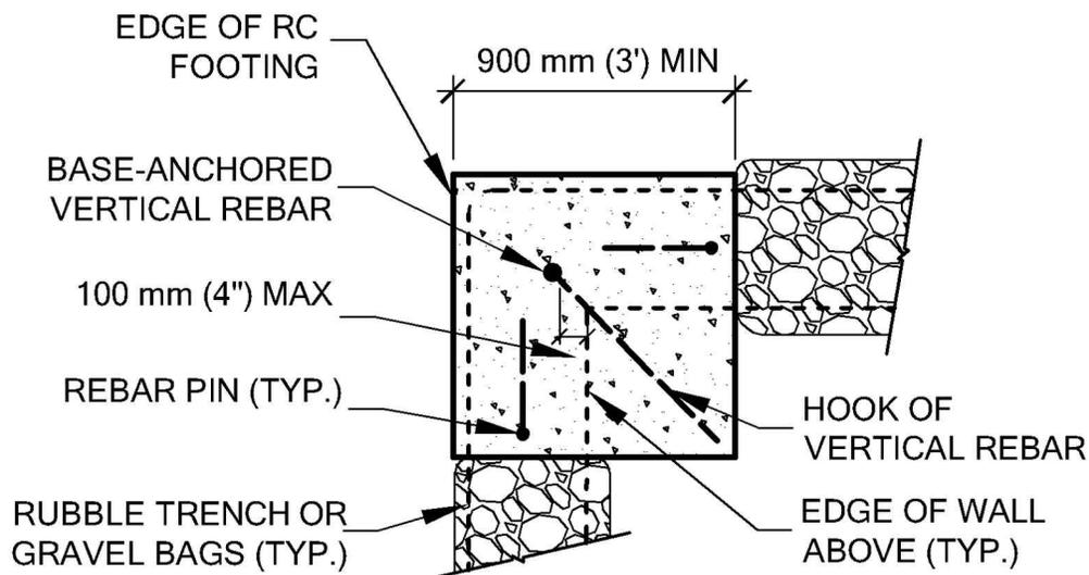
Figure 6: Spot footing to anchor long vertical rebar extending to the bond beam.
