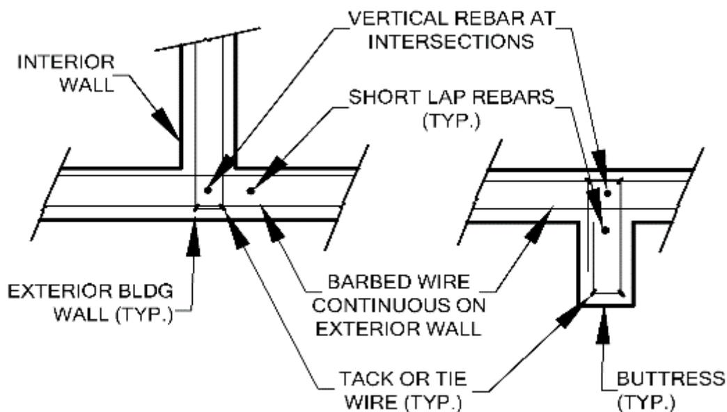
Figure 9 Barbed wire continuous along walls (right to left): a- runs across adjacent wall, b- runs across wall to end of buttress and returns.
