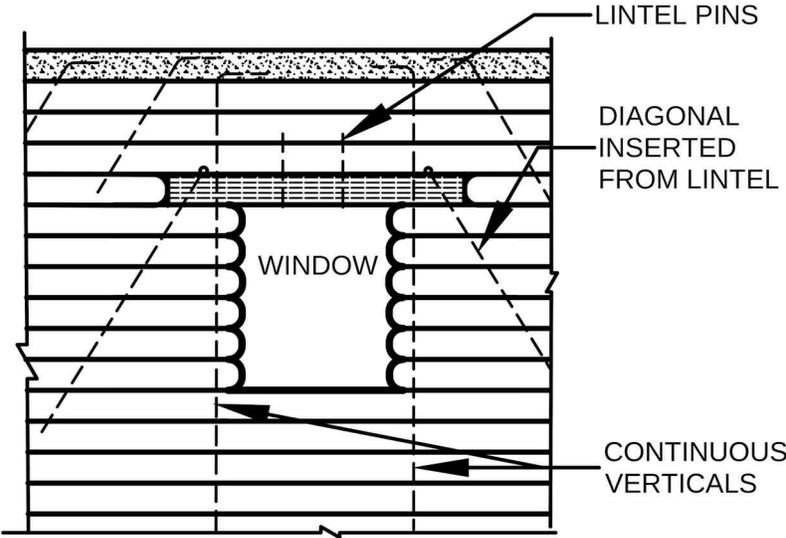
Figure 16: Wide wall openings can have strong connections to bond beams.
