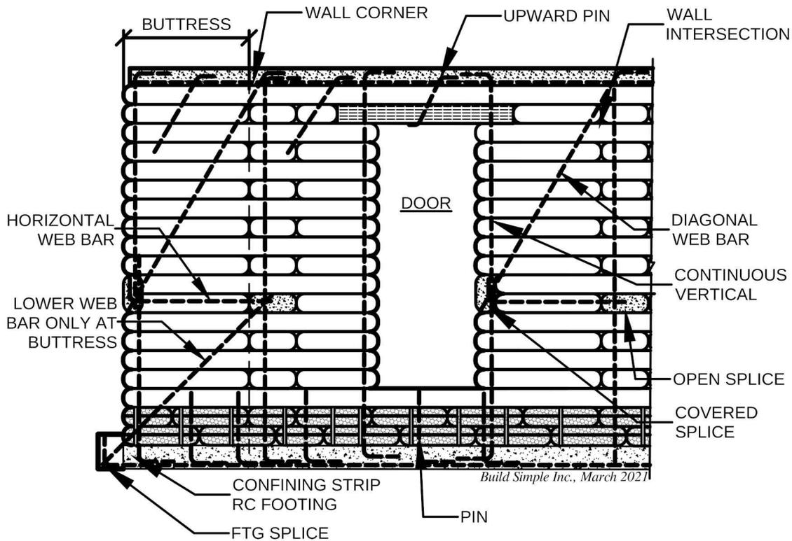
Figure 19: Full wall height rebar truss assemblies can be built with high strength CE footings.
