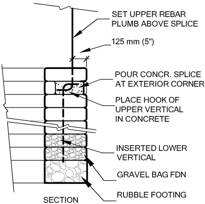
*Figure 12: Connect verticals with hooks in one-course high open splice.*
