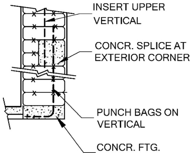
Figure 14: An upper rebar inserted into a splice two courses high.
