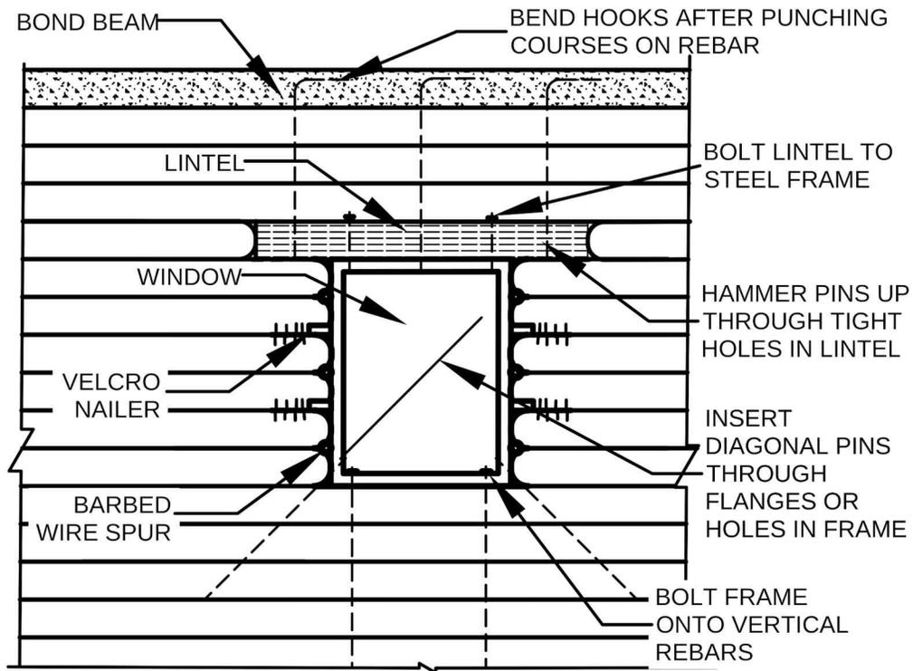
Figure 20: Welded steel frame connected to lower and upper rebars use velcro nailers and rebar spurs to connect into wall material on both sides.
