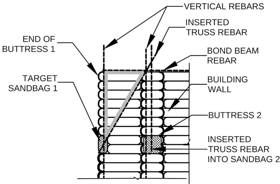
Figure 15: Standard grade reinforcement uses triangular bracing at external corners or buttresses.
