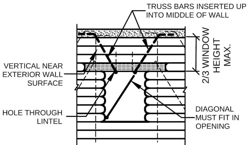
Figure 18: Diagonals connecting lintels to bond beams.
