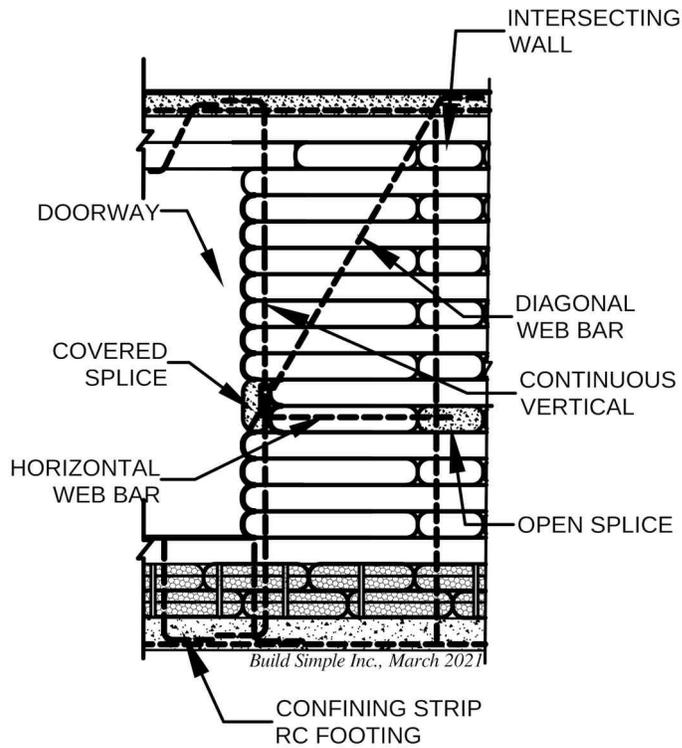
Figure 17: High strength CE can use single or double braces near doorways or corners.
