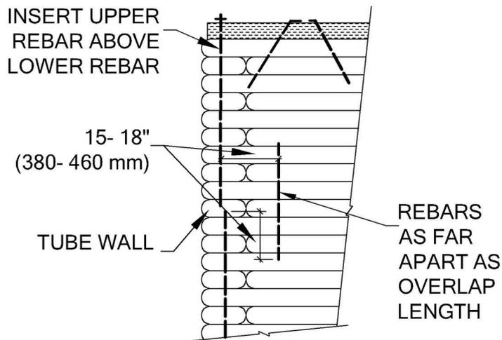
Figure 10: Improved overlapped inserted rebar technique uses a distant lap rebar.
