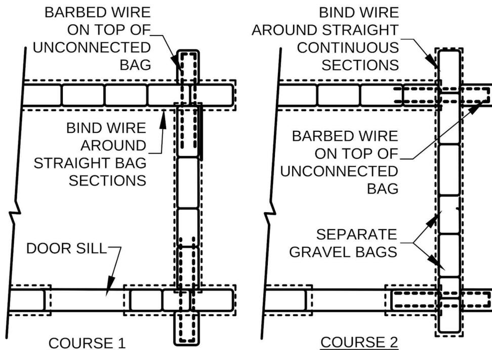
Figure 5 Bind gravel bag courses (right to left): a- Wrap straight sections excepting openings; b- Alternate laying wire on bags unconnected with binding wire from course to course.
