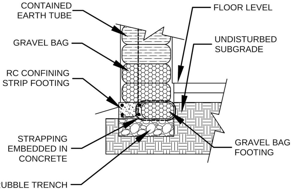
Figure 7: Confining strip footing holds gravel bags in place with modest concrete use.
