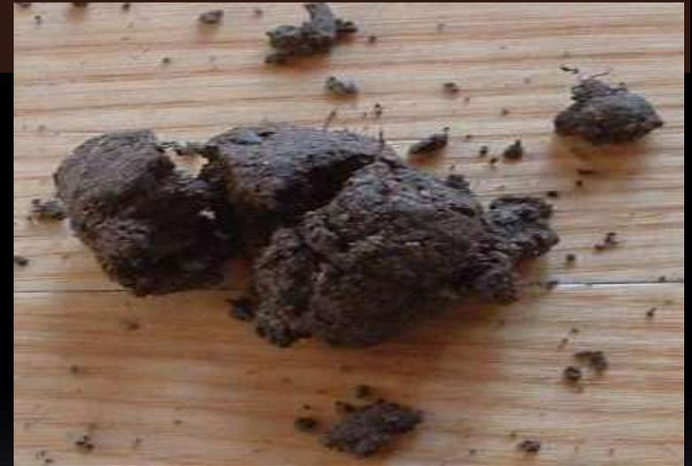
Too wet: leaving a wet spot, cracking
