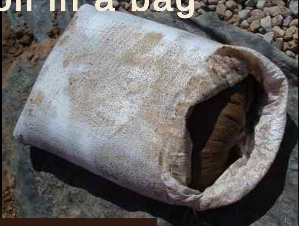
**Soil masses that break when lifted 24 hours after tamping are weak soil**
