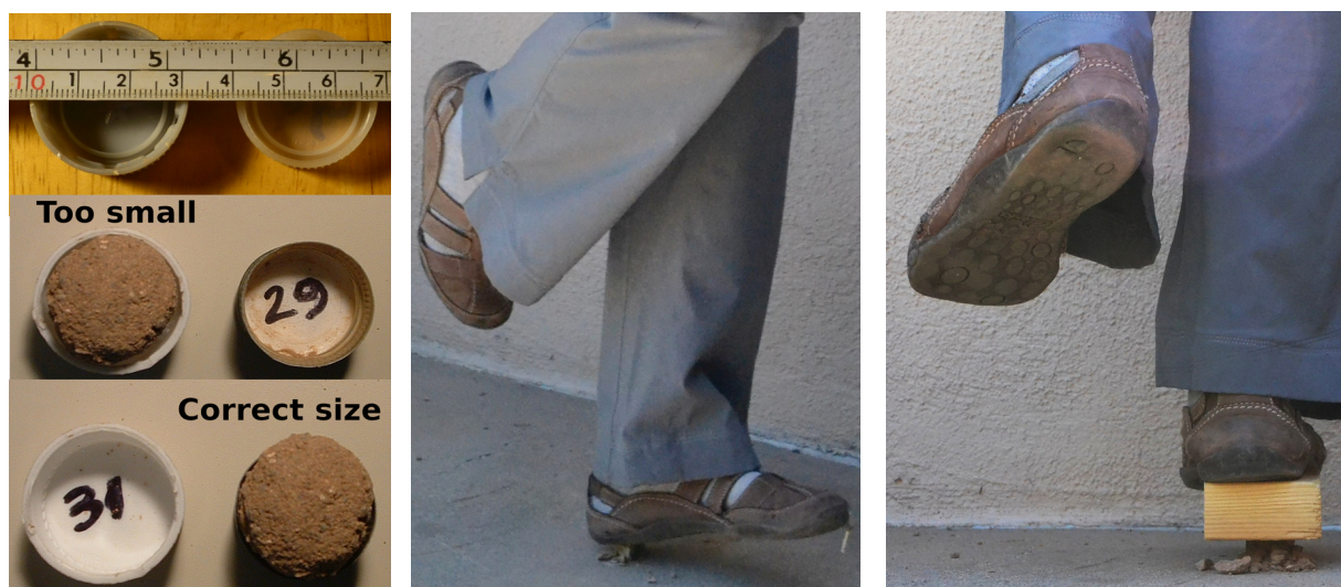
Figure 9 Crush balls underfoot (left to right): a- Use 30 mm balls only; b- balance on a ball; c- Put a piece of wood on a strong ball to retest.
