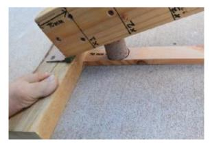
If the hinge board is thicker than the samples are high, good! Find a thin piece of wood the right thickness to make the lever board level on the sample. Draw on it to locate the sample accurately each time.
