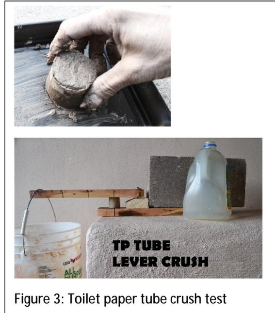
Figure 3: Toilet paper tube crush test
