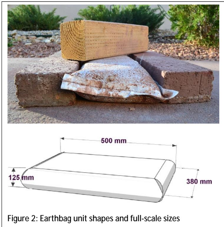
Figure 2: Earthbag unit shapes and full-scale sizes
