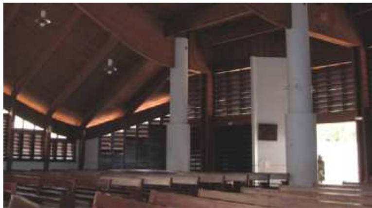
Even if wood is not chosen for structure or walls it can be used for breathable wooden louvers, shutters, or railings. Ask older people in the villages which local woods are more durable. Wood can also be smoked to discourage termites and mold.
