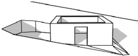
Rain will need to run around and away from building walls. Rain always flows downhill, so on the uphill side a building needs a small swale or ditch that will direct the water away.
