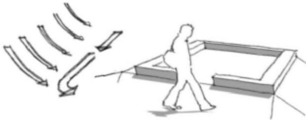
Have the land slope down away from the building on all sides. On the uphill side it might only slope down 10 cm in 3 m (4" in 10'). In humid climates locate the swale at least 3- 6 m (10- 20') from the building.
