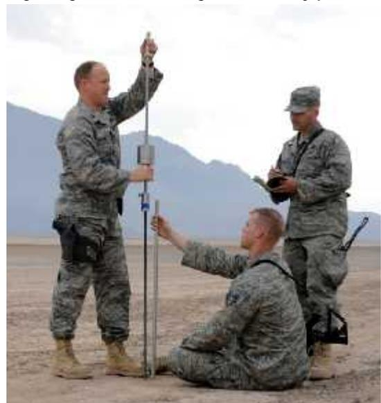
Contractors can make a standard penetration test (SPT) with a 65 cm (25.5") long piece of pipe and a 63.5 kg (140 lb) slide hammer. It evaluates deeper soil layers well. The SPT is best for sandy soils. It may be less accurate for clay and gravelly soils, but can assess them if laboratory tests are not available.
