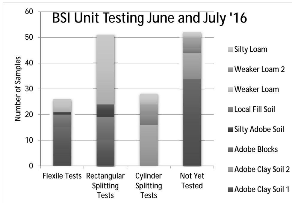
Some of these tests have been used to develop a series of four soil mixes of sequential strength. Soils of different but known strengths are critical to upcoming research.
