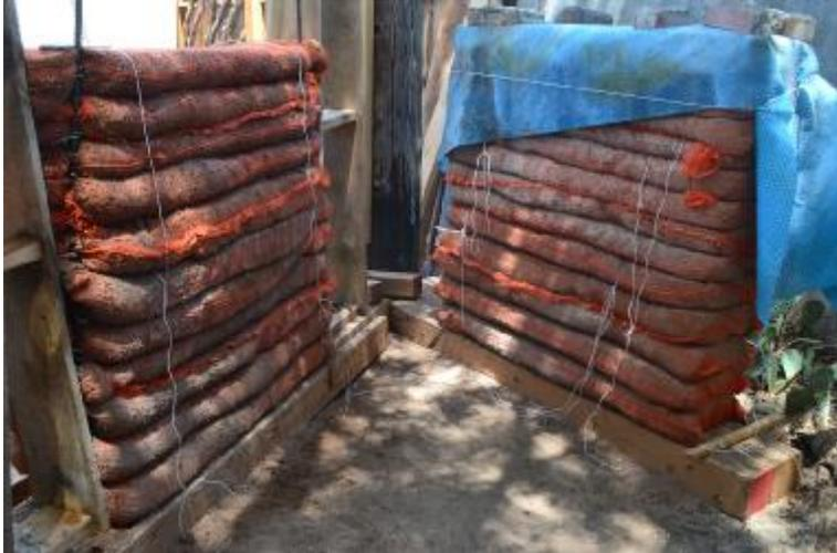
Three 16 sf solid (mesh tube) wall samples (two in photo at left) have been curing since mid-June. One has no reinforcement or barbed wire, another has standard barbed wire and inserted rebar, and the third has barbed wire attached to anchored, exterior rebar. These shear tests will provide needed strength and yield point and elasticity information for the different reinforcement levels.
