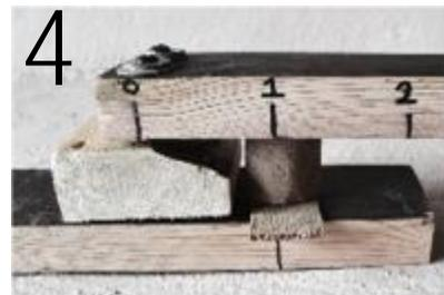
The lever plank must be level when you start the test. If your sample is not tall enough, set it on a piece of wood or shingle (photo 4).
