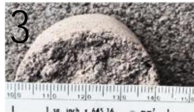
Measure the widest and narrowest directions of any oval tops. Write down the average of the two measurements.
