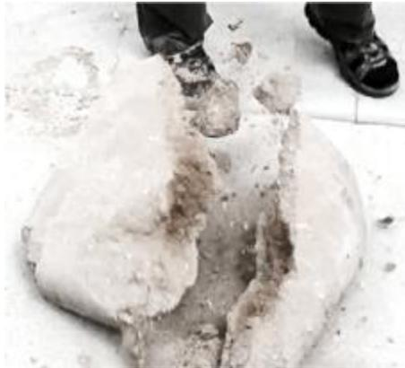
A sample passes the test if no more than 4"/ 100 mm breaks off any corner, and it does not break in half.
