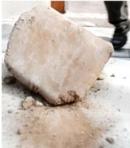
Below left: This sample passed because it stayed whole and less than 4"/ 100 mm broke off the damaged corner
