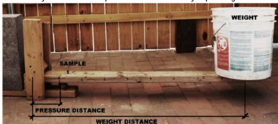
force on the sample will be 6 x the weight. The total weight for your test includes weight you place on the lever board- and *HALF THE WEIGHT OF THE LEVER BOARD*.
