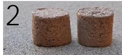
Measure the diameter of the top of each sample (in photo 3 this sample is 41 mm diameter). Metric is easier than inches for accuracy. Discard any larger than 43 mm or smaller than 39 mm.
