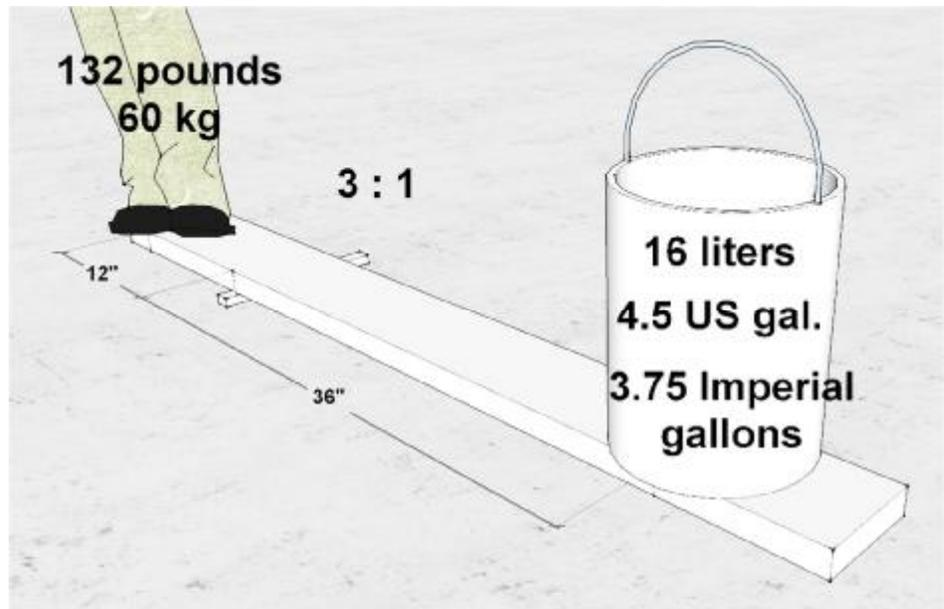
The tester stands on the 12" mark on the short side of the board. Place a bucket of water centered over the 36" mark.
