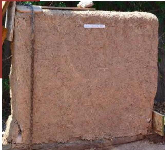
Despite the small scale and their inability to convert acceleration readings to displacement, these small shake tests showed that adding buttresses to a corner reduced motion by 26%. Adding a solid mass between 2 buttresses at the corner reduced motion by 33% and prevented damage to the wall. Using Solidworks software for FEM analysis, considering the barbed wire barbs as independent pins allowed a modeling accuracy of  $\pm 1.5\%$ .
