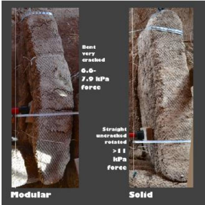
*Above: BSI tests of 60% scale wall corners compared walls solidified between courses with modular construction (not solidified between courses)*
