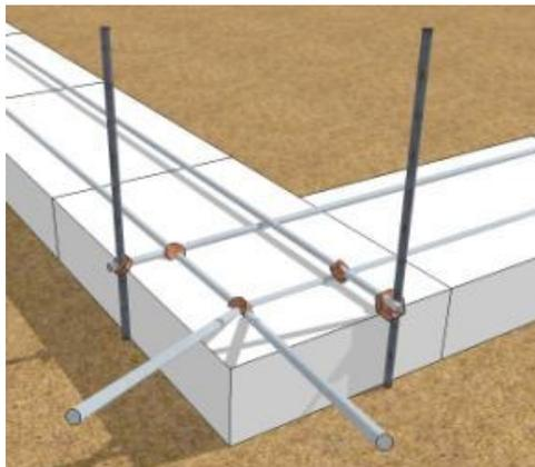
Reinforcement can include half lengths of rebar hammered into moist walls. Better yet, barbed wire can be attached to whole rebars spanning from the footing to bond beam at wall and buttress ends.
