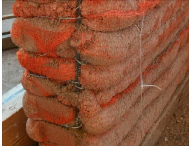
*Right: BSI test wall of solid CE with barbed wire attached to anchored exterior rebar.*
