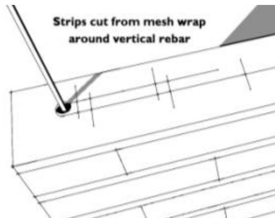
*Right: Mesh strips of 5.3 mm (4 ga) welded wire mesh on 15 cm (6") centers for New Zealand*
