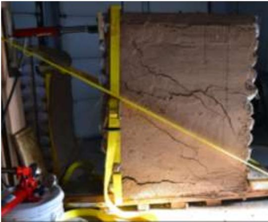
Right: Modular CE of solid-weave bags built between anchored rebar
