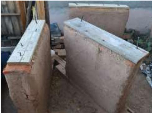
Solid contained earth (walls built in mesh tubing that uses fill damp enough to solidify between courses, aka hiperadobe) is stronger than conventional modular contained earth. Modular contained earth is the conventional technique that has courses separated by solid woven fabric and joined only by bonds between the barbed wire and the cured bag fill.
