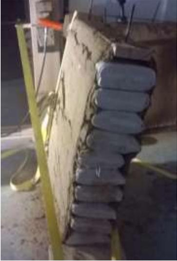
The walls of strong soil resisted in-plane forces well but repeatedly twisted out of plane during testing. It was remarkable that neither of the walls overturned, although at times reaching as much as 15 degrees twist and a significant slope.
