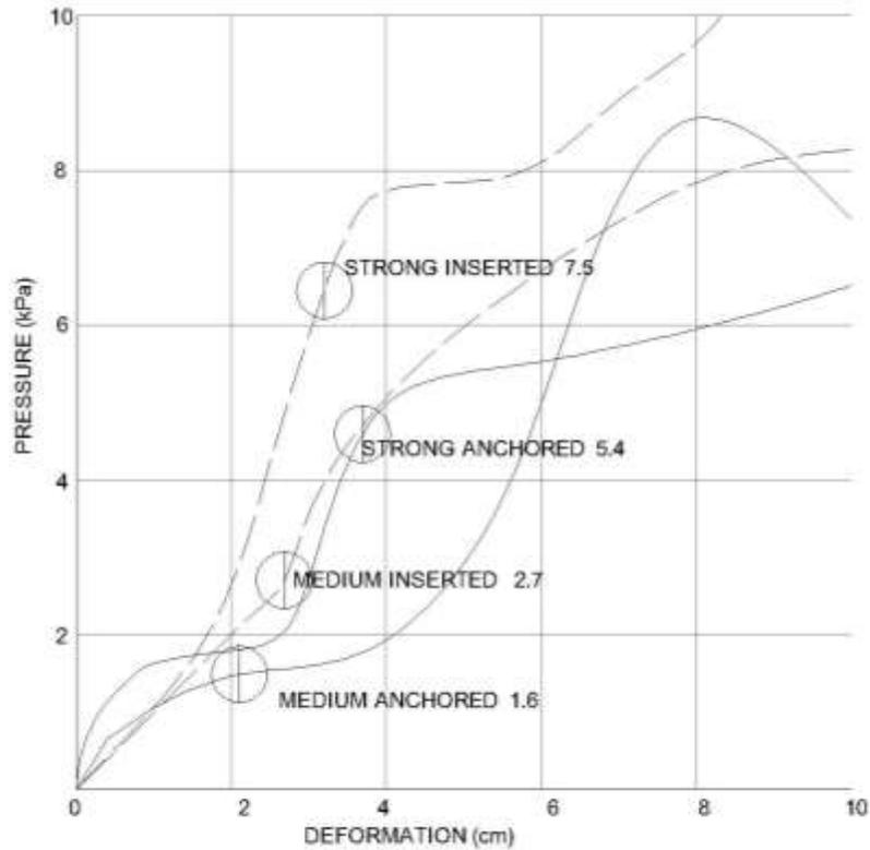
**CONTAINED EARTH SHEAR STRENGTH AT FIRST CRACK**
