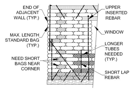
Figure 14: Bags limit rebar integration with wall material even when mixed with short tubes.
