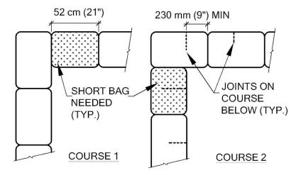
Figure 3: Use shorter bags near corners and intersections for good running bond bag overlaps.
