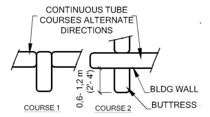
Figure 24: Continuous tubes and barbed wire unite walls to piers (left to right): a- Midwall buttress; b- Corner buttress tube layout.
