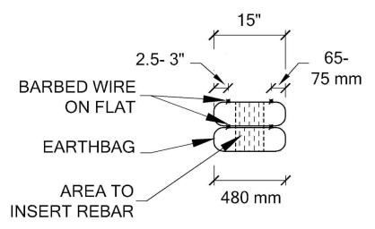
Figure 4 Barbed wire location on the flat course top near rounded course edges.
