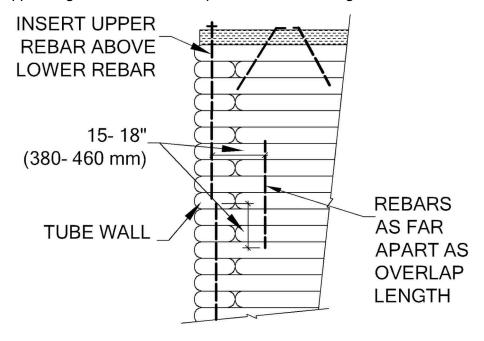
Figure 27 Improved overlapped inserted rebar technique uses a distant lap rebar.
