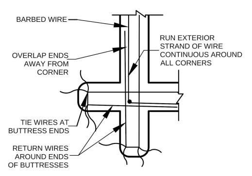
Figure 25: Run external strand of barbed wire continuous around building and use interior strands to unite buttress to building walls.
