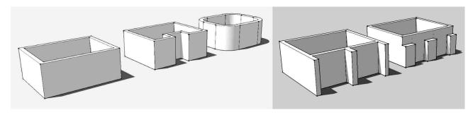
Figure 7 Structural wall elements (left to right): a- Corners on a rectangular building; b- Extra corners for nooks; c- Curved walls; d- Buttresses extending from walls; e- Piers that thicken walls.
