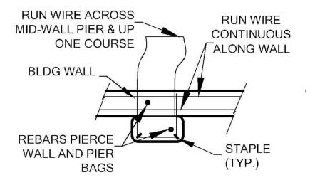
Figure 17 Barbed wire on piers should use a loop of wire woven to the next course.
