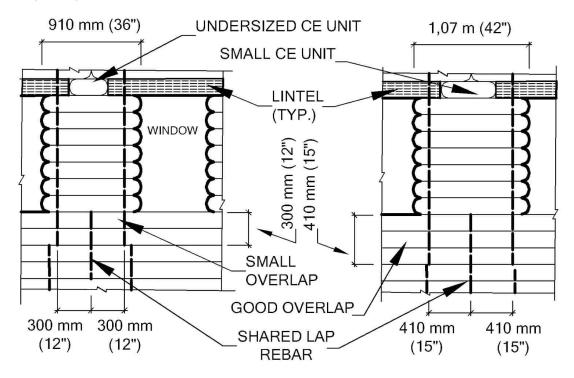
Figure 28: Spaced lap rebar dimensions (left to right): a- Minimum distance; b- Better distance.
