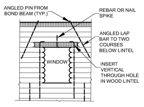
Figure 30: Vertical rebars adjacent to a window opening connect to the lintel.
