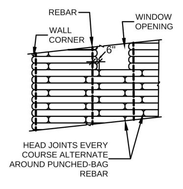
Figure 19: Punched-bag technique needs tubes starting on alternate sides of a vertical rebar to allow good overlap of tubes between courses.
