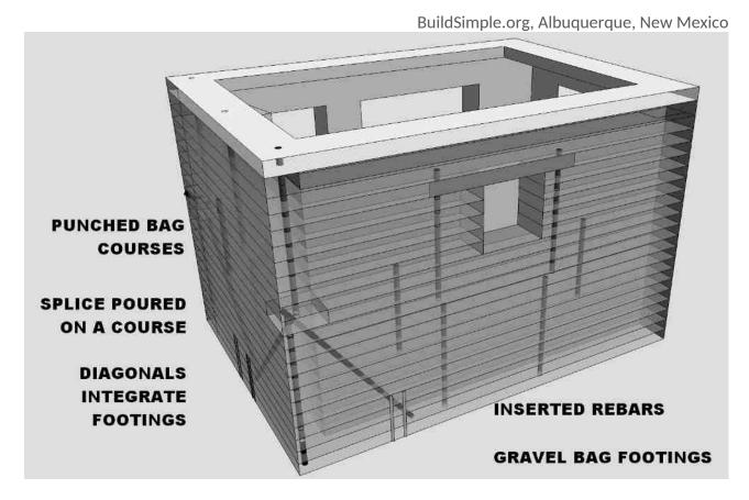
Figure 1: Strengthen corners by interconnecting upper and lower rebar to diagonals with a concrete splice poured during wall construction.
