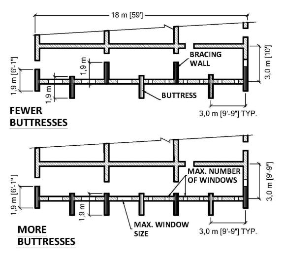
Figure 8 Bracing panels (above to below): a- A long supported right to left wall with few buttresses needs doorways far from wall corners; b- More buttresses allow doors closer to the supported wall.
