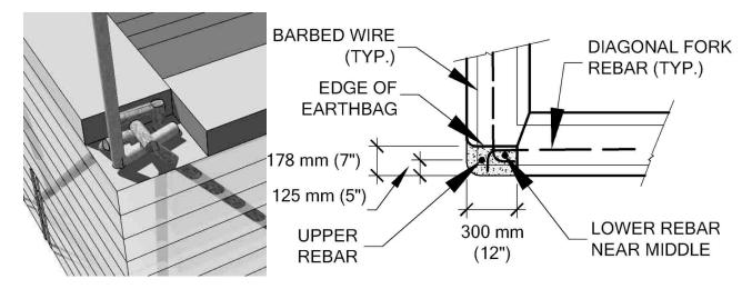
Figure 23 Spliced forks: a- hooks overlap at corner; b- Minimum size for a fork open splice.
