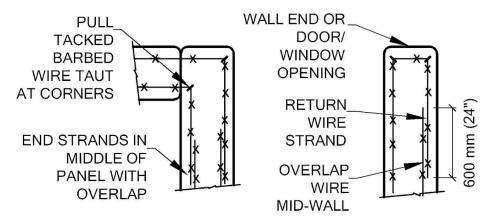
Figure 5 (left to right): a- Always run barbed wire continuous around corners and locate strand ends in middle of walls; b- Run barbed wire around wall end or opening edge and return.
