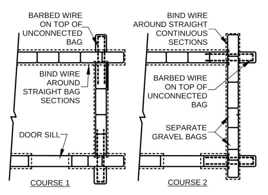
Figure 12 (left to right): a- Always bind the straight wall section that crosses a pier or intersecting wall first, then bind shorter sections next; b- Include buttresses in binding on alternate courses.
