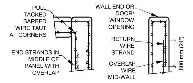
Figure 5 (left to right): a- Always run barbed wire continuous around corners and locate strand ends in middle of walls; b- Run barbed wire around wall end or opening edge and return.
