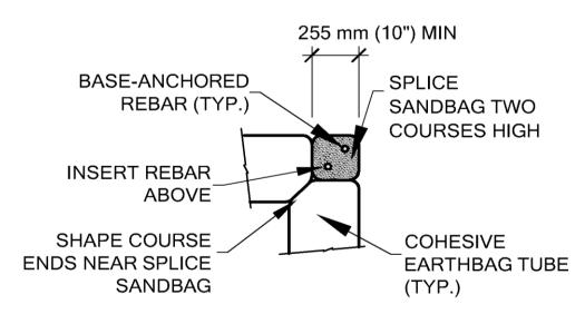
Figure 12 Covered splice sandbag location at mid-story height of external wall corners.
