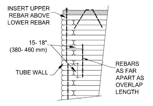
Figure 31 Improved overlapped inserted rebar technique uses a distant lap rebar.
