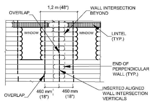
Figure 32: Use greater distance between openings when the area includes a perpendicular wall.
