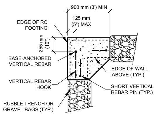
Figure 11 Spot footing to anchor short vertical rebar that will use an open splice.
