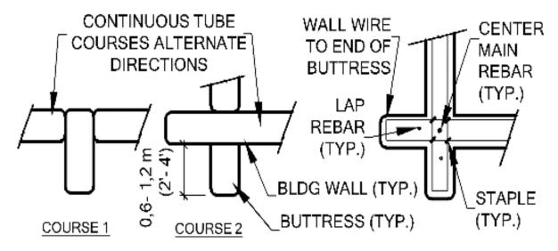
*Figure 23: Continuous tubes and barbed wire unite walls to piers (left to right): a- Mid-wall buttress; b- Corner buttress tube layout; c- Corner buttress barbed wire and rebar.*
