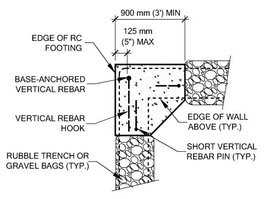
Figure 13 Spot footing to anchor short vertical rebar that will use a covered splice.
