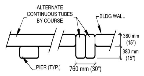
*Figure 21 Piers integrated to the wall (left to right): a- Continuous tube lengths along the wall; b-Every other course interrupt the wall to run tubes across the pier and the wall.*
