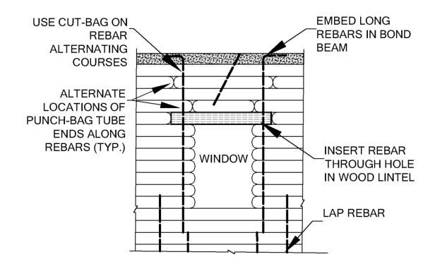
*Figure 33: Vertical rebars adjacent to a window opening connect to the lintel.*
