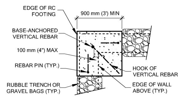
Figure 10 Spot footing to anchor long vertical rebar extending to the bond beam.
