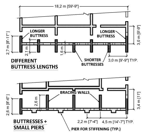
Figure 9 Examples of bracing panel sizes at different bracing line distances (above to below): a-Different buttress lengths to maximize rooms with 3 m (9'9") bracing line distances; b- Wider 4,5 m (14'- 9") bracing line distances used with stiffening piers between bracing panels.
