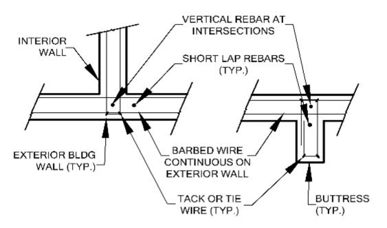
Figure 20 Barbed wire with both strands of barbed wire continuous along walls (right to left): a- At wall intersections run wire across adjacent wall, b- At buttress run wire across wall and return.
