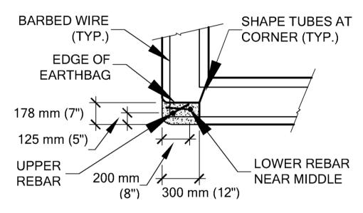
Figure 27 Use a narrow gap for an open concrete splice to connect upper and lower rebars.
