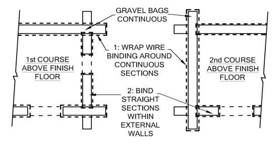
Figure 15 (right to left): a- Bind around gravel bag courses; b- Pull taut and attach wire at overlap with a nail through both strands, then hold it in place by wire wrapped around the strands.
