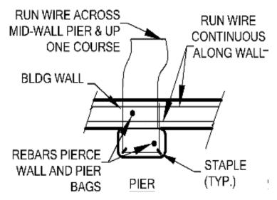
Figure 22 Barbed wire on piers should use a loop of wire woven to the next course.
