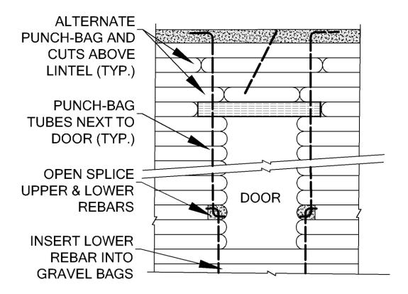
*Figure 34: Splice vertical rebars next to doorways to provide vertical rebars extending below the door sill.*
