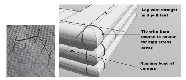
Figure 35 Add strength where barbed wire turns corners (left to right): a- Pins cut from wire mesh and bent can pierce upper and lower courses, b- Tie wire from bends in barbed wire out both sides and up to the next course.
