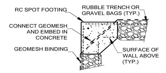
*Figure 9 Geomesh embedded in spot footings at corners can confine adjacent gravel bag footings.*
