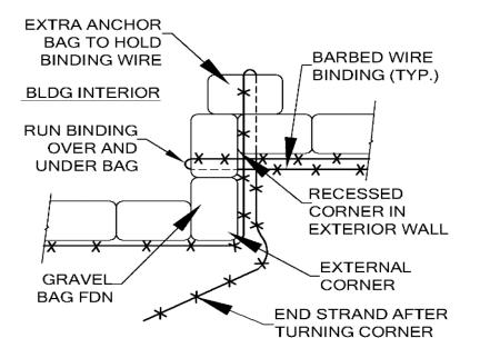
Figure 16 Start barbed wire at recessed corners by wrapping strands around a perpendicular bag.
