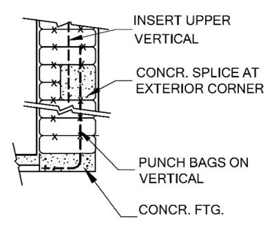
Figure 28 An upper rebar inserted into a covered splice bag two courses high, then the sandbag is emptied and filled with concrete.
