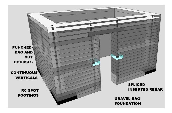
*Figure 1: Strengthen corners with vertical rebar that is base-anchored in spot reinforced concrete footings. Insert spaced lap rebars at other locations on gravel bag foundations.*
