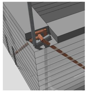
Spliced forks can also add strength to buttresses or piers.
