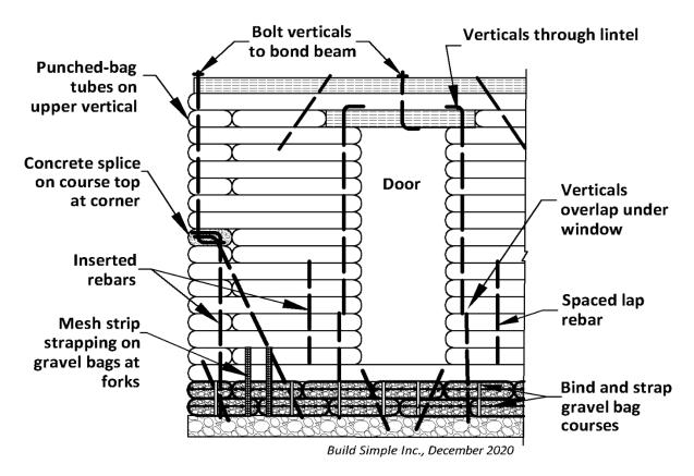
Figure 6: Improved reinforcement system for low seismic risk areas requires little Portland cement.
