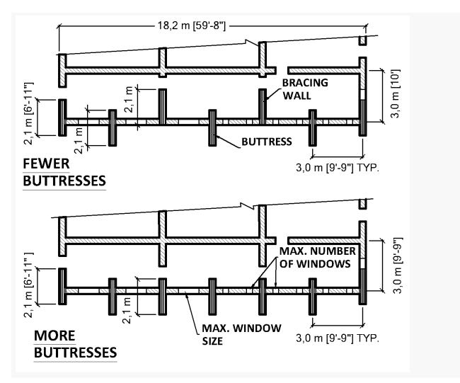
Figure 8 Examples of bracing panel sizes at 3 m (9'9") bracing line distances (above to below): a-Few buttresses and doorways distant from wall being braced; b- More buttresses and doorways closer to wall being braced.
