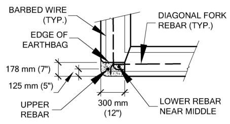
Figure 38 Reinforcement locations in a fork splice.
