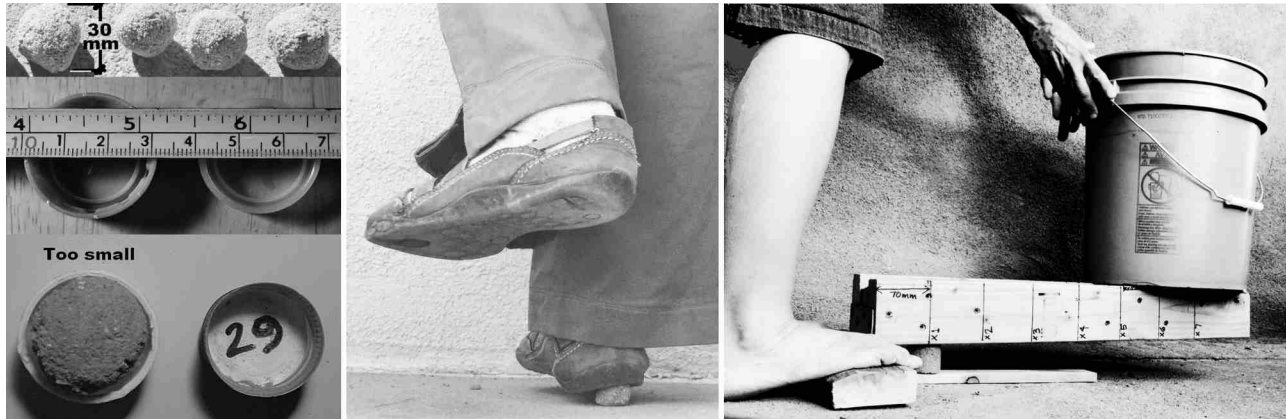
Figure 3 Estimating soil strength with small samples (left to right): a- Small balls can be compared to measured bottle caps to check for accurate size; b- Small soil balls can be crushed underfoot; c- Samples made in toilet paper tube forms can be crushed under a bucket of soil on a small wooden lever.
